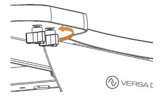
Pick up the keyboard surface. Align the slots on the side brackets to meet the loosened thumb screws on both the left and right sides. Gently slide the keyboard tray brackets into the gap between the thumb screws and the top surface.
