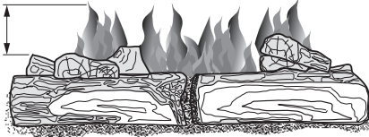
Figure 30 - Correct Burner Flame Pattern with Control Knob Set to HI (5)
