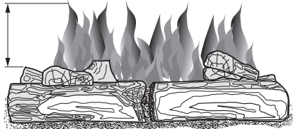
Figure 31 - Incorrect Burner Flame Pattern with Control Knob Set to HI (5)
