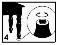
Some furniture comes with height adjustment knobs underneath each leg. To lower or to raise each leg, you need to turn clockwise or counterclockwise, respectively.
