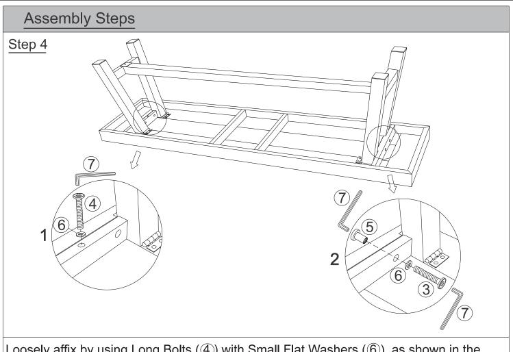
Loosely affix by using Long Bolts ((4)) with Small Flat Washers ((6)), as shown in the picture (1) and Middle Bolts ((3)) & Small Flat Washers ((6)) with Sleeve Nuts ((5)), as show in the picture (2). Tighten with using the Allen Key ((7)).
