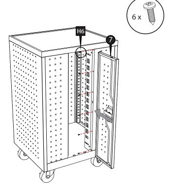
Attach the left and right front doors (8 & 9) to the assembly with 12 screws (H6).
