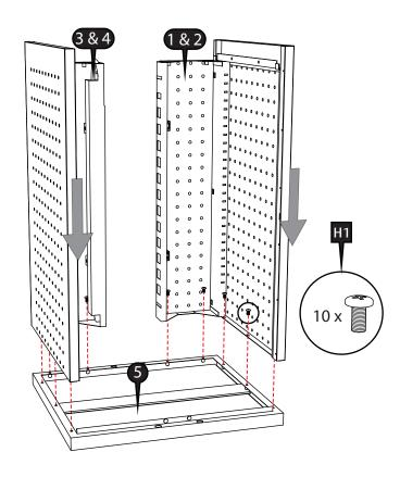
Place the bottom panel (6) onto the assembly. With a light force, secure into place.
