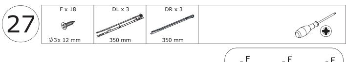
Fix runner(DL) and (DR) to plate 16 and 17 respectively with screw(F) as shown.
