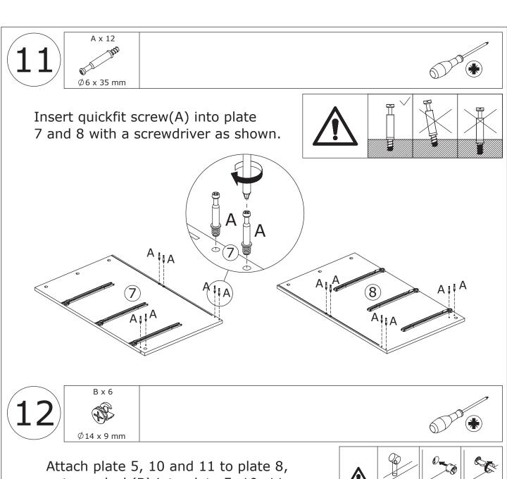
put cam lock(B) into plate 5, 10, 11 and turn clockwise to tighten as shown.
