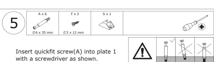
Fix part(S) to plate 1 with screw(F) as shown.
