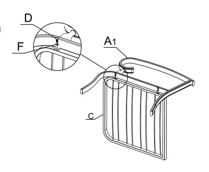
Loose attach all connections at the beginning, adjust alignments then fully tighten all joints
