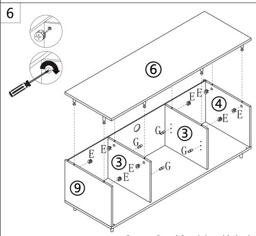
Connect Board 6 and the table body, then twist Screw E to the board as displayed. Insert Part E into the holes in both Board 3.
