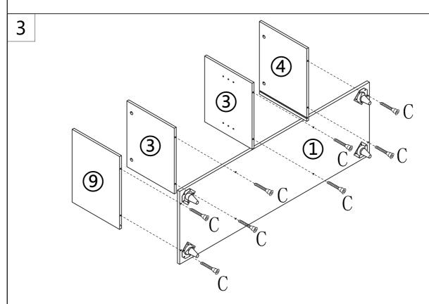
Twist Screw C to connect Board 9, 3, 4 to Board 1 as displayed.
