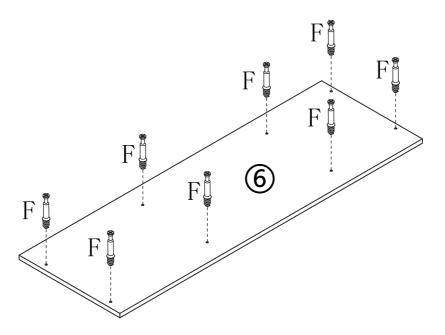
Twist Screw F into the white holes in Board 6.
