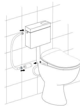
Water from the exposed cistern
