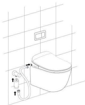
Water supply next to the toilet
