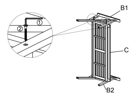
With assistance from your adult partners, turn the Chair into the other side Repeat the same process of step 2 to secure Left Leg Panel (B1) with Seat Panel (C) by using Screw (2) and Allen Key (1)
