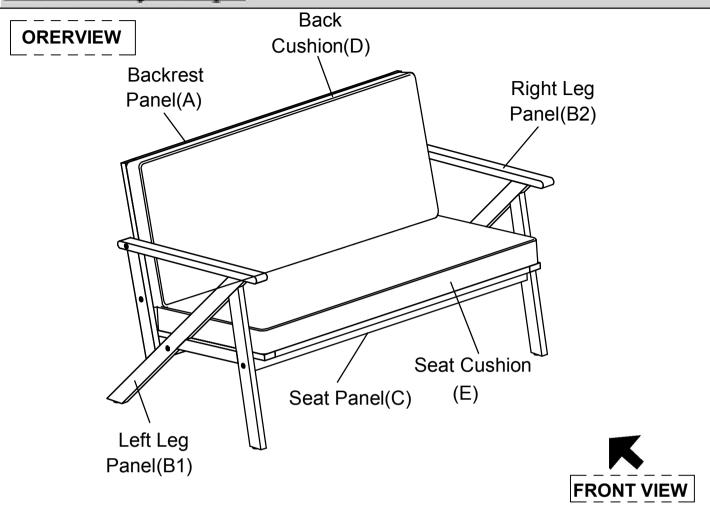
This Loveseat has multiple parts and may require up to some 30 minutes to assemble. To give you an overview of the Loveseat, the above picture is to help you put the various parts into perspective. Please read through the instructions here below to familiarise the parts and steps before assembly.
