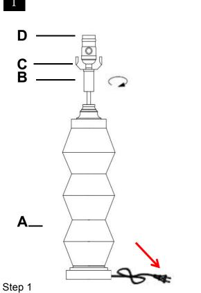
Pull power cord to connect the Neck (B) to the Base (A). Screw the Neck (B) onto the Lamp base (A) Be careful not to twist the power cord and tighten securely
