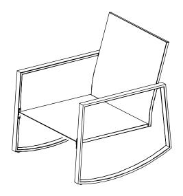
• Attach the seatback (A) and the seat base (B) using a M6 x 35 socket head cap screw (E) with a flat washer (G). Do this in two places.
