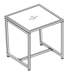
Flip the assembly upside down. Attach the table top (J) and the legs(K) using a M6x35 socket head cap screw (E) with a flat washer (G). Do this in four places.
