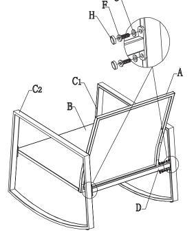
Completly assembly, then fix and tighten all the screws. Finally place the screw covers (H) over them.
