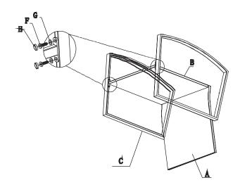
Flip the assembly upside down . Secure the arm rests(C&D) to the seat base (B) using M6 x 20 screws (F) with a washer (G). Do this in four places.
