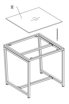
Completly assembly, then fix and tighten all the screws. Finally place the screw Covers (H) over them.
