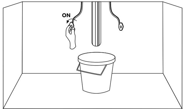
10. Proceed to sink drain installation. Once the drain is installed, turn the faucet on for approximately 60 seconds. Check for any leaks. Test both hot and cold water to ensure they are running properly.
