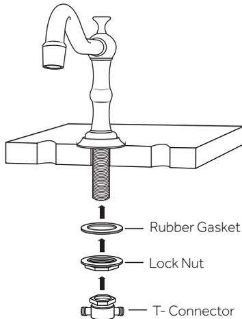
4. Remove the lock nut, metal washer, and rubber gasket from the valve stem labeled 'cold.' Insert the stem into the faucet hole on the right.
