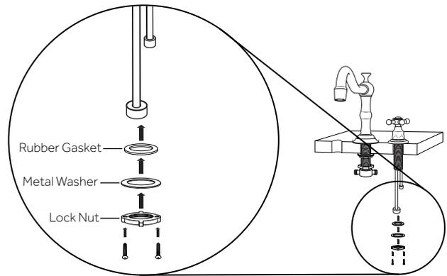
6. Repeat steps 4 and 5 for installing the 'hot' valve stem into the left faucet hole.
