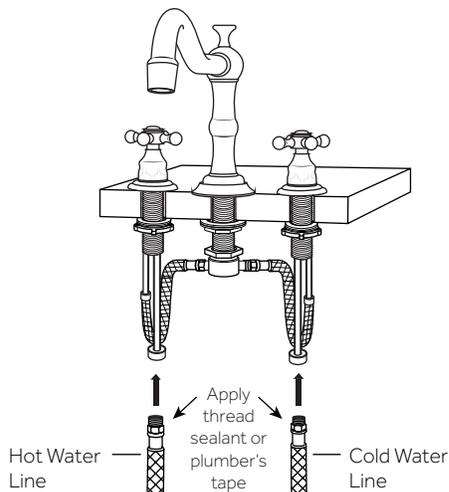
9. Once installation is complete, turn the main water supply back on. Check for any leaks underneath.
