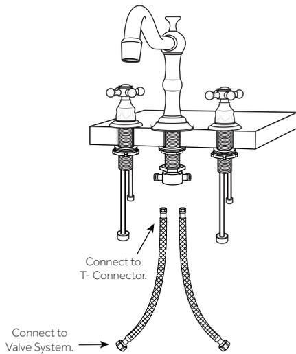
8. Attach the main water lines to the valve stems. Use an adjustable wrench to tighten, but be careful not to overtighten. Apply thread sealant or plumber's tape to each threaded connection. Ensure that you are connecting the hot and cold lines accordingly.
