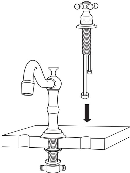
5. From under the counter, slide the rubber gasket back onto the valve stem followed by the metal washer. Secure to the counter by hand-tightening the lock nut. Finish securing by tightening the screws on the lock nut using a Phillips screwdriver.
