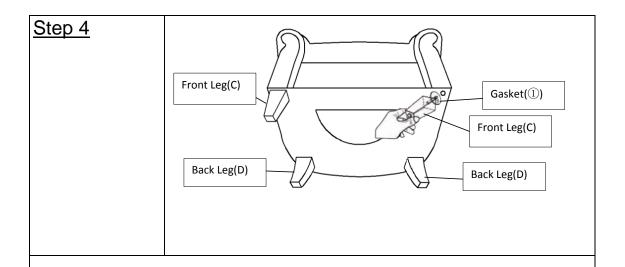
Install Front Leg(C) into the Chair Base(B) by putting a Gasket(1) on the threaded stem. Then insert the threaded stem into the mounting position at the corner of the bottom of Chair Base(B).
