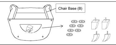
Place the Chair on its back on a clean, non-marring surface as pictured above. Carefully unzip the pouch at the bottom of the Chair Base(B) and remove the Front Leg(C), Back Leg(D) and Hardware.
