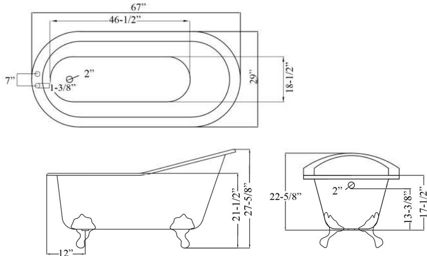
Dimensions of fixture are nominal and may vary within the range of tolerances established by ANSI Standard A112.19.1M. Dimensions and specifications subject to change without notice.
