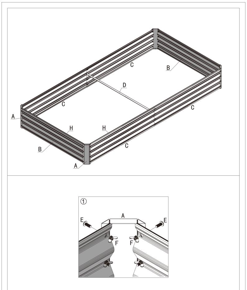
1 Attach 2 Corner Connectors #A to 1 Short Sheets #B with 8 screws #E, and secure with 8 wingnuts #F .
