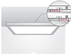
STEP 6: Lift fixture up against bracket. Align the arrow sign ▼ from bracket to unlock-sign from fixture. Slide to locked-sign
