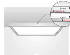
STEP 4: Slide safety wire into slot of bracket. Rest product on safety wire while doing eletrical installation. Do not disconnect safety wire
