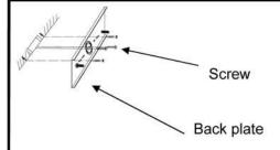
Attach the back plate to the junction box.
