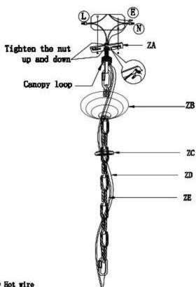
IMPORTANT: Test sockets with bulb before dressing the fixture.
