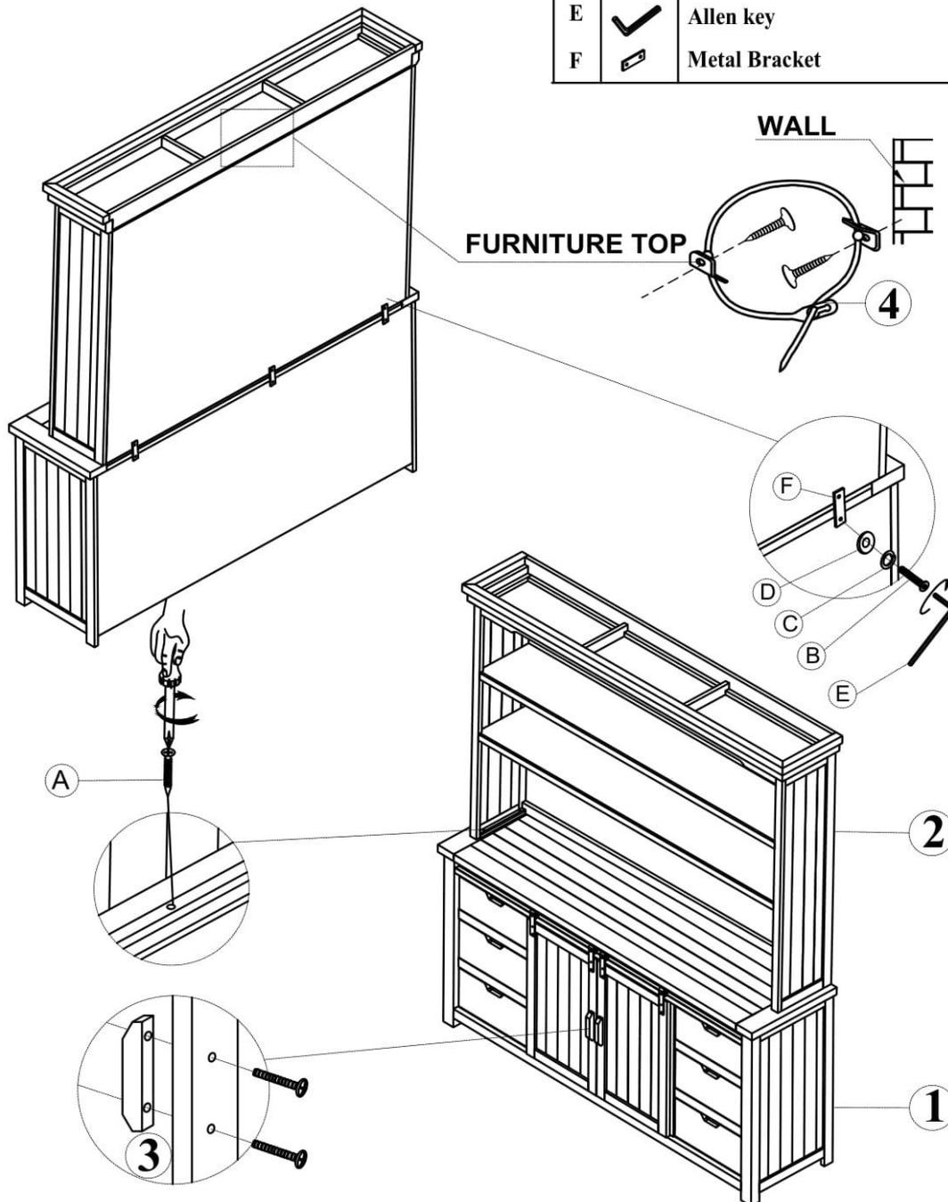
PLEASE NOTE : To help prevent the possibility of tip-over. Install the ANTI- TIP OVER restraint provided.
