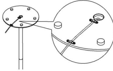
Push the heater head onto the top hollow tube and fix it in position using the supplied 2 X M4\*8 screws.
