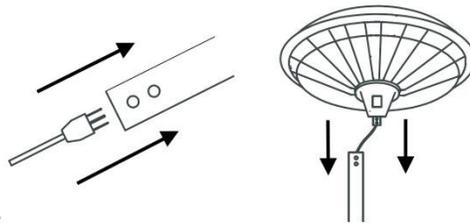
Pull the power cord gently out of the base as much as possible. Fix the power cord under the weighted base using the supplied 4pcs M4 nuts.
