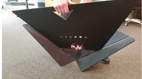
Squeeze Panels 1 and 2 inwards. Slide Panel 3 into long slots of Panel 1 and 2
