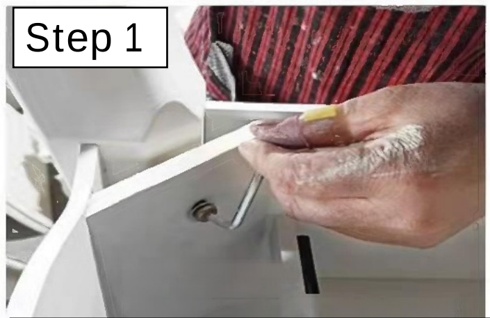
Step 1 Install the legs using an Allen wrench and screw number one
