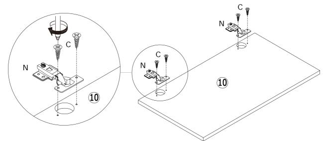
Fix hinge(N) to board 10 with screw(C) as shown. Attach door 10 to board 8 by fixing hinge with screw(C) as shown.
