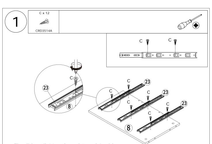
Fix slide rail 23 to board 7 and 8 with screw(C) as shown. Please pay attention to the holes where the accessories are inserted.
