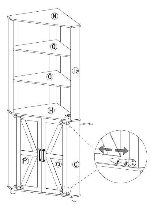
If there is a large gap after the installation of the door, please twist the screw of the door hinge back halfway and move the door left and right.
