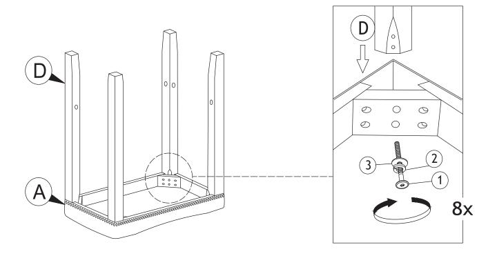
Do not tighten the hardware completely!
