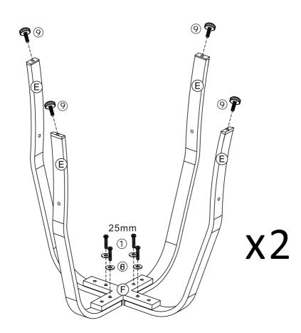
Screw on the part F with four Adjusting Screws (9).
