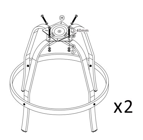
Adjust alignments and NOW TIGNTEN ALL SCREWS with wrench (40) with Allen key (11).
