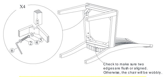
Put the chair on a flat level surface to make sure the chair is level and then tighten fully the all bolts.
