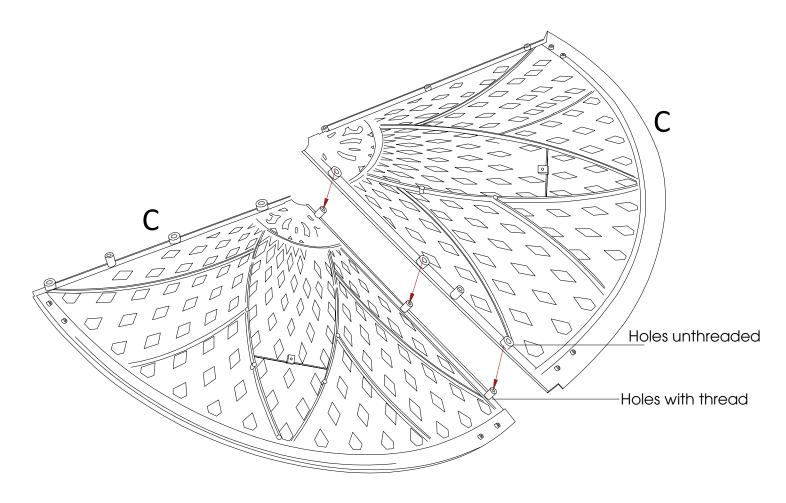
Then, attach the third TABLETOP with the holes aligned as shown in the diagram below. Same as the Step1.
