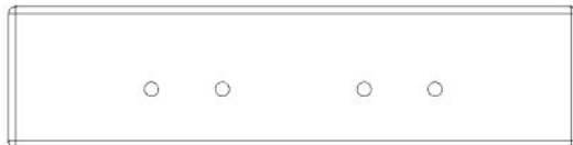
DB2 - DRAWER BACK BOARD - W4L20012 (x1) 5/8"x2 3/8"x9 1/2" (16x60x241)
