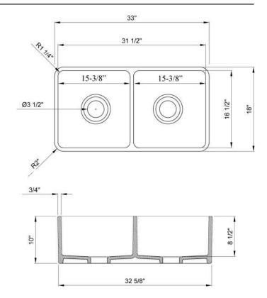
Dimensions of fixture are nominal and may vary within the range of tolerances established by ANSI Standard A112.19.2. Dimensions and specifications subject to change without notice.
