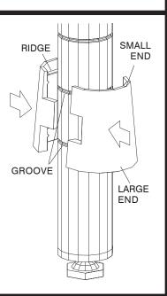
3 Stand a (D) Shelf on end, and from the BOTTOM side of the shelf (the bottom side is recessed), slide the TOP end of a post through a corner hole until the half-sleeves are seated in the corner hole. Repeat with remaining posts.
