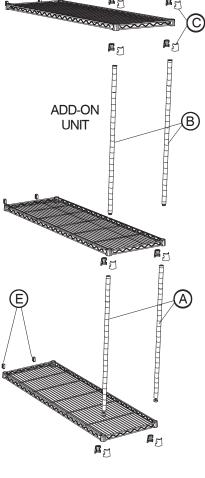
To build the four corner posts, screw the (A) Lower Posts (with levelers) onto the (B) Upper Posts (with plastic caps). Hand tighten.
