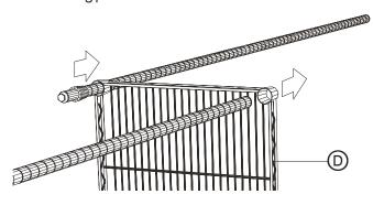
Set unit upright. Press shelf firmly at each shelf corner, close to corner holes until firmly seated.
