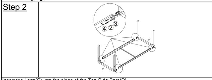
Insert the Legs(C) into the sides of the Top Side Bars(D).
