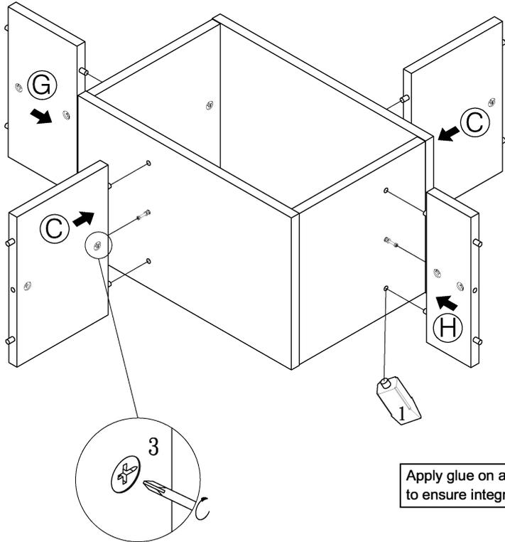
Apply glue on all wooden dowels to ensure integrity of the structure.
