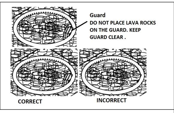
To ensure proper function, the Guard (02) on the Burner (1) should never have lava rocks (A) covered over it.
