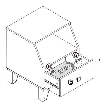
Extend the two outer slides of the runners so that they could align with the sides of the drawer.
