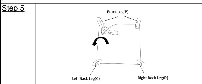
Finally, seal the Dust Cover back on to the underside of the Seat(A) and smooth the edges by hand.
