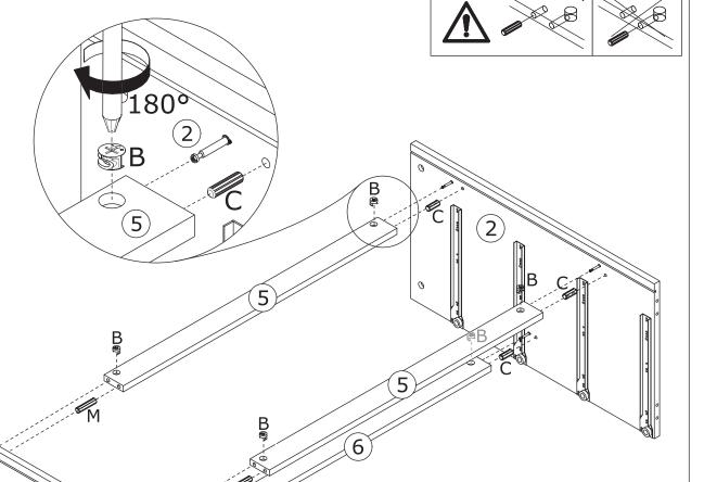
Connect board 2 and 4 to board 5 and 6, add cam lock(B) into board 5,6 and turn clockwise to tighten as shown.
