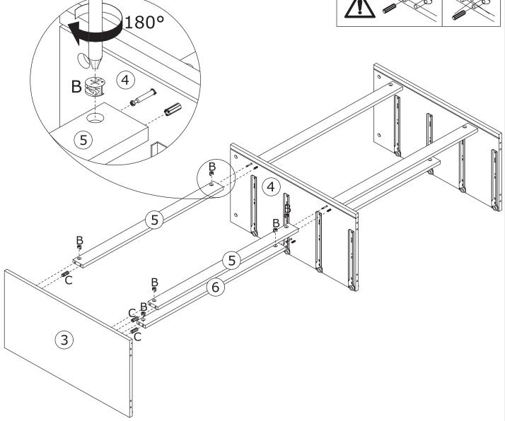
Insert SHORT wooden dowel(C) into board 3 at first.
