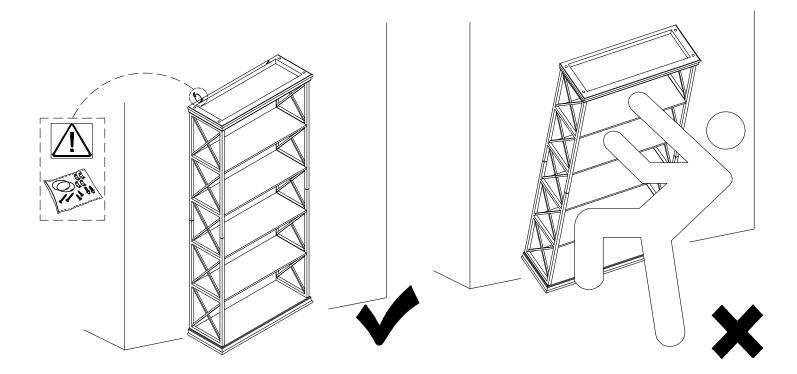
( Install tip-over restraint provided) Use of tip-over restraints may only reduce but not eliminate, the risk of tip-over.
