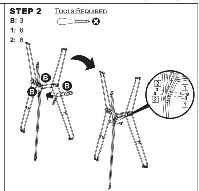
As indicated in the drawing, align three Upper Supports (B) with the top of Legs (A) and secure using six M6x25mm Screws (1) and six M6 Nuts (3).
