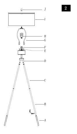
Step2 Insert the Harp (G) into the Saddle (E). Put the shade(I) on the Harp(G),then tighten the Finial (J)into the Harp (G)
