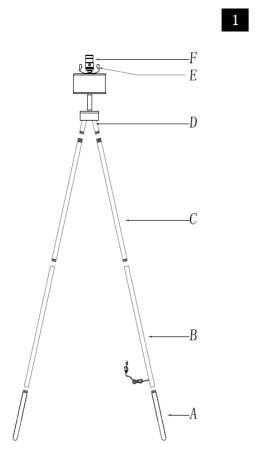
Step 1 Make sure all parts could be aligned before assemble Do not rotate lamp body too hard avoid base screm broken Fasten tube(C) onto tube(D). Fasten tube(B) onto tube(C) Pull cord through tube(B) to tighten stem(B.C.D) connections, Insert the bulb(H) into the socket(F). Fasten tube(A) onto tube(B).
