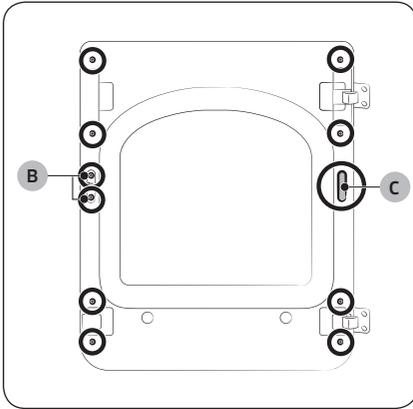
10. Remove the **hole cover (C)**, and then insert and tighten the glass holder using the removed 10 screws.
