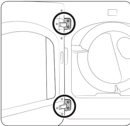
12. Reinstall the door on the front frame, and then carefully insert and tighten the 4 hinge screws.
