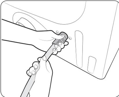
4. Connect the angled end of the water hose to the filling valve at the bottom of the rear frame. Turn the coupling manually until it is tight.
