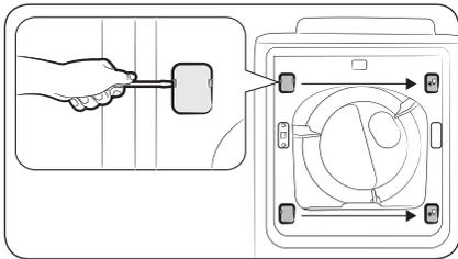
6. Use a flat-head screwdriver to remove the two hinge covers from the original side. Install the hinge covers on the opposite side as shown.
