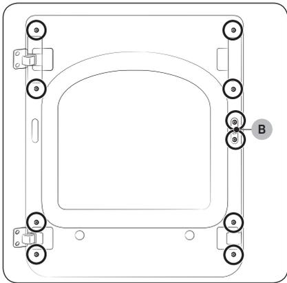
7. Locate and remove the 10 screws as shown. Note that **screw B (x2)** is longer than the others.
