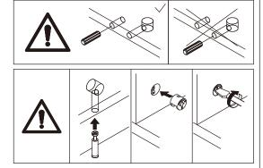
Insert wooden dowel(B) into board 12 at first.
