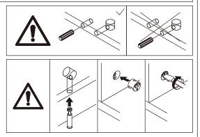
Insert wooden dowel(B) into board 5 at first.
