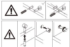
Insert wooden dowel(B) into board 7 at first.
