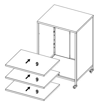
Install component 9 to the position shown in the diagram
