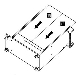
Assemble the combination of panel no. 4, 5 & 15 to the unit by using Crosshead Screw m6.3 x 40mm (A17). Use Allen Key (N1) to tighten the Crosshead Screw m6.3 x 40mm (A17).
