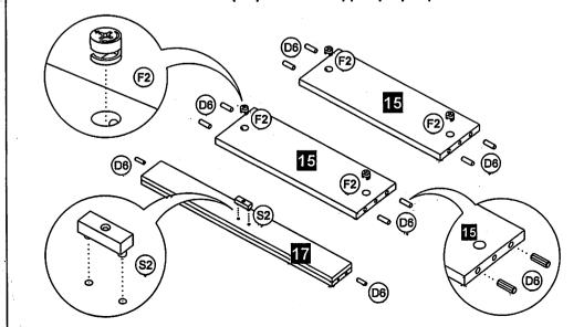
STEP 8 Insert Mini Fix Cam (F2) & Mini Fix Bolt (F2) at panel no. 4 & 5. Insert Wood Dowel (D6) at panel no. 4 & 5.
