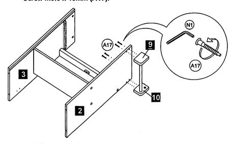
Assemble the panel no. 13 to the unit by using Crosshead Screw m6.3 x 40mm (A17). Use Allen Key (N1) to tighten the Crosshead Screw m6.3 x 40mm (A17).
