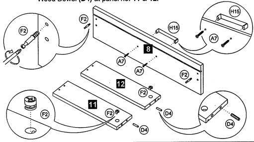
STEP 2 | Assemble the panel no. 11, 12 & 16 together by using Screw (A10).
