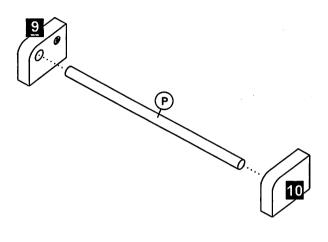
STEP 11 Insert the Hanging Steel Pipe 18mm x 377mm (P) into the large marking hole between the panel no. 4 & 5. Use Mini Fix 15mm (F2) to assemble all panels below together.
