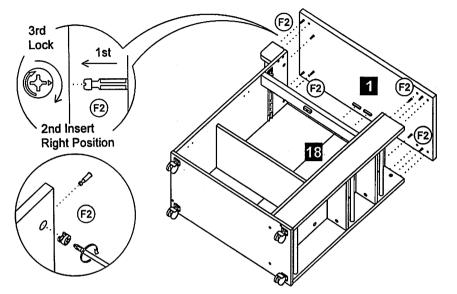
STEP 18 Assemble the Single Plastic Cap (R2) by using Screw (A2) to secure the panel no. 18. Use Nail (N3) to secure the panel no. 14 & 18.
