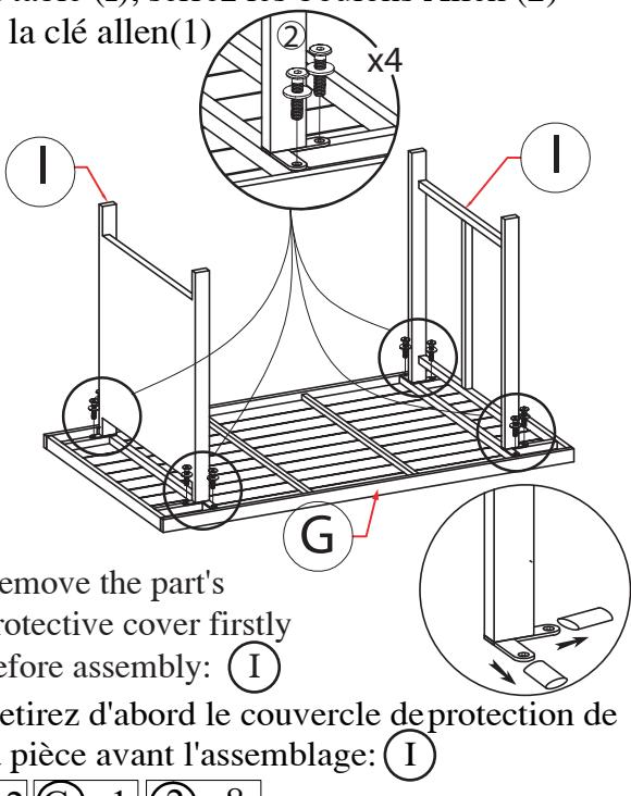
⚠ Remove the part's protective cover firstly before assembly: (I)
