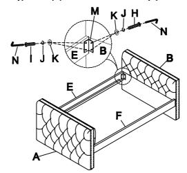
2 ATTACHED BACK REST(C), LOCK WASHER(J), FLAT WASHER(K), BOLT(G), BY ALLEN WRENCH(N).
