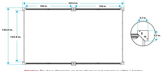
Attention: The above dimensions are manually measured and error is within 1-2 inches. We suggest you anchor the gazebo after installed the main frame.
