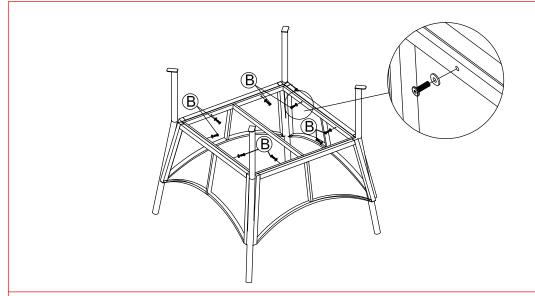
STEP 5 : Connect The Part from Step 4 with Bolt (B),Flat Washer (D) with Allen Key (E).
