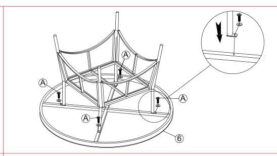
STEP 6 : Connect The Part from Step 5 and Table Top (6), tighten Bolt (A), Flat Washer (D) with Allen Key (E).
