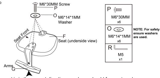
Note: Make sure the armrest is in the correct direction, overhang should face outwards.
